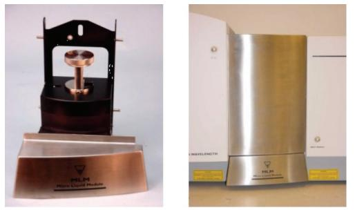
The MLM measures the entire sample in the instrument by circulating the sample with a stir bar. The amount of sample needed depends on its size and concentration. Prior sample preparation is often needed to achieve proper dispersion (see APPENDIX B, *Sample Handling* for more information on how to disperse samples) in order to obtain accurate and valid results.
