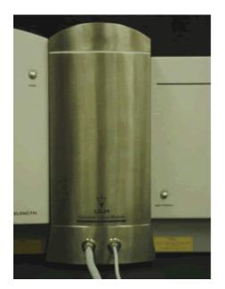
The ULM measures the entire sample introduced to the instrument by re-circulating the sample. The amount of sample needed depends on its size and concentration. Prior sample preparation is often needed to achieve proper dispersion (see APPENDIX B, *Sample Handling* for more information on how to disperse samples) in order to obtain accurate and valid results.
