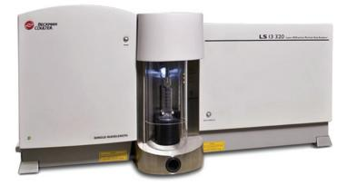
The LS 13 320 consists of an optical bench and five different sample handling modules:
